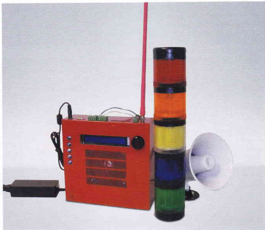
The SAM receiver may be used as a standalone installation or may be supplemented with external sirens and visual threat-level indicators.
